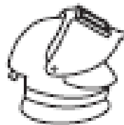
Class 7D Respirator facepiece with loose-fitting hood or helmet for radiation protection
