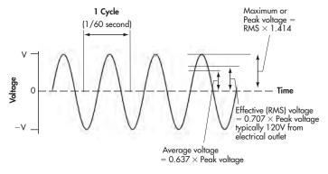
Any variation to the voltage waveform, in magnitude or in frequency, is called a power line deviation. However, not all power line deviations result in disturbances that can cause problems with the operation of electrical equipment.
