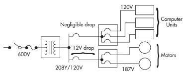
An even better approach is to effectively create a new supply system for the sensitive loads by using a transformer in addition to a separate feeder
