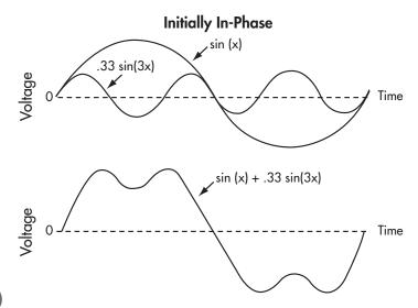
In this example, the two waveforms begin in-phase with each other, and produce a distorted waveform with a flattened top. The composite waveform can be changed by adding the same harmonic, initially out-of-phase with the fundamental, to obtain a peaked effect:
