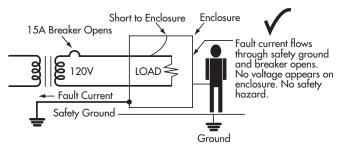
If the equipment were properly bonded and grounded the equipment enclosure would present no shock hazard and the ground fault current would effectively operate the over-current device.
