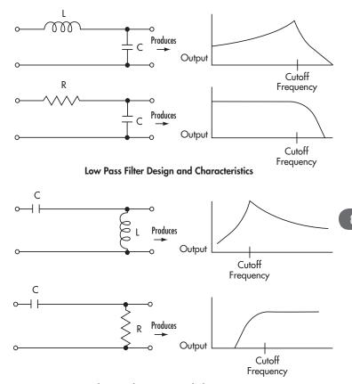
High Pass Filter Design and Characteristics
