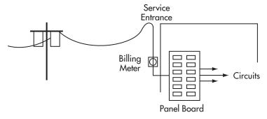
In larger distribution systems this power panel board will supply other panel boards which, in turn, supply circuits.
