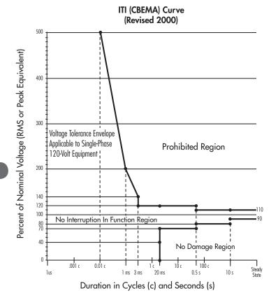
The susceptibility profile implies that computers can tolerate slow variations from -13% to + 5.8%, and greater amplitude disturbances can be tolerated as their durations become shorter. In fact, many computers can run indefinitely at 80% of their nominal supply voltage; however, such operation does lead to premature wear of the power supply.
