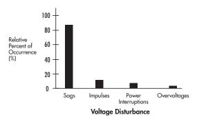
Figure 23: Relative Occurrence of Disturbances to Power Systems Supplying Computers
