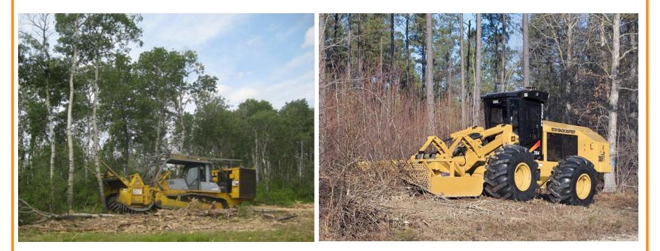
Drum-style mulcher used for tree clearing
