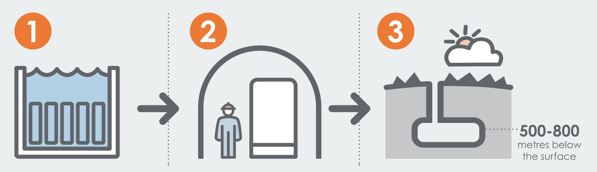
Used fuel comes out of the reactor and is placed in wet storage for cooling.
