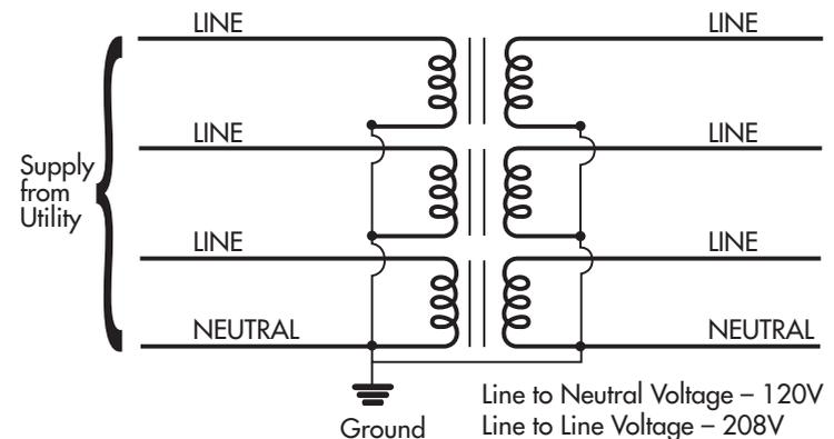
Typical voltage levels for three phase power supply are 120 V/208 V, 277 V/480 V (in the United States and Canada) or 347 V/600 V (in Canada).
