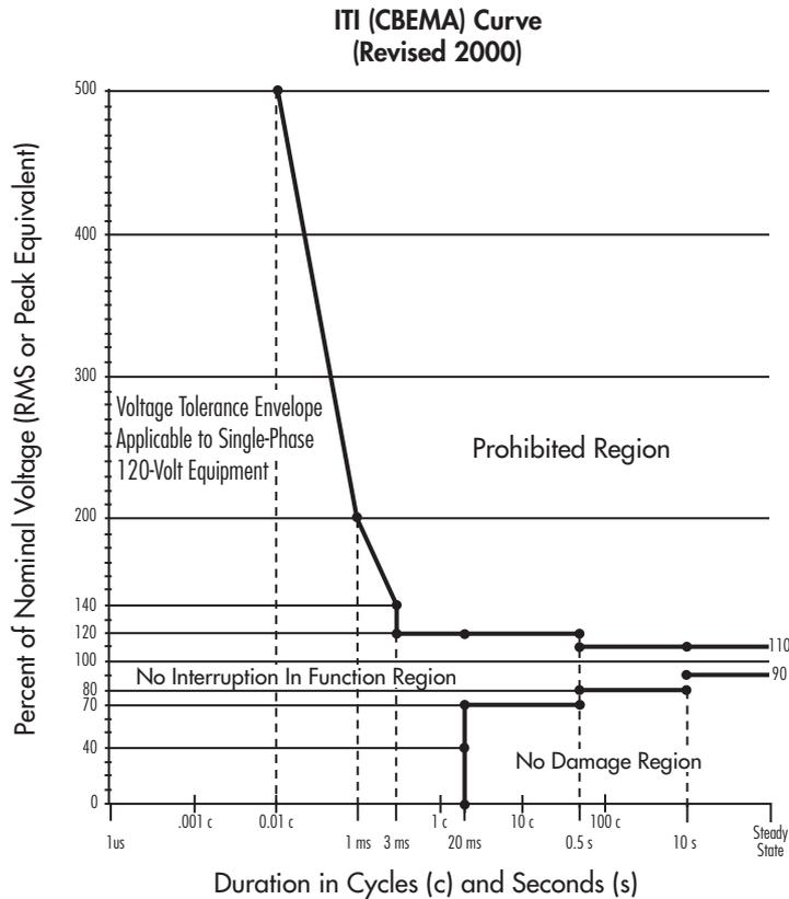
The susceptibility profile implies that computers can tolerate slow variations from -13% to + 5.8%, and greater amplitude disturbances can be tolerated as their durations become shorter. In fact, many computers can run indefinitely at 80% of their nominal supply voltage; however, such operation does lead to premature wear of the power supply.
