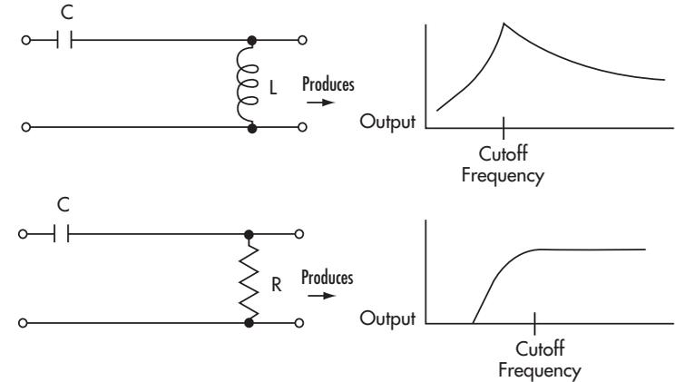
High Pass Filter Design and Characteristics
