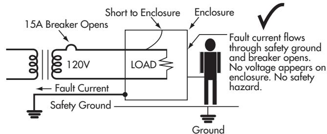
If the equipment were properly bonded and grounded the equipment enclosure would present no shock hazard and the ground fault current would effectively operate the over-current device.
