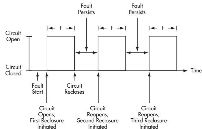
Normally a few seconds are required to clear a fault and energize the appropriate circuitry for a reclosure. The reclosing interval for a recloser is the open circuit time between an automatic opening and the succeeding automatic reclosure. In the above diagram, three intervals of duration 't' are indicated.
